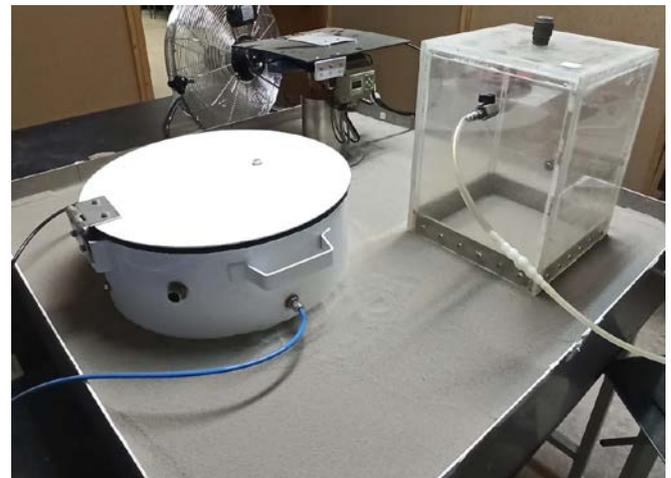
Figure 2.1: Typical configuration experiment with different radon flux systems.
