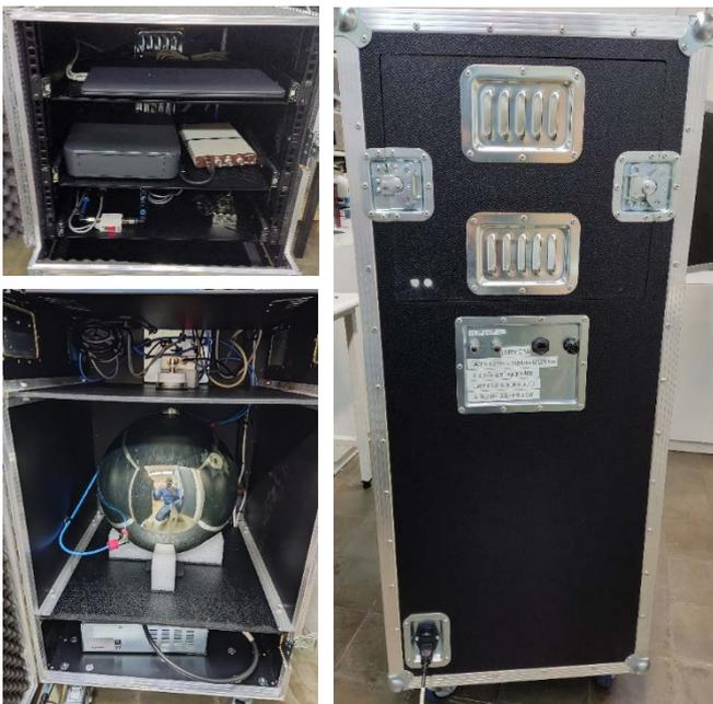
Figure 1.1: inside (left) and back (right) of the new ARMON monitor. In the inner trays, from top to bottom: i) laptop; ii) datalogger and multichannel analyser; iii) sensors and voltage transformers iv) amplifier v) detection volume vi) high voltage power supply.
