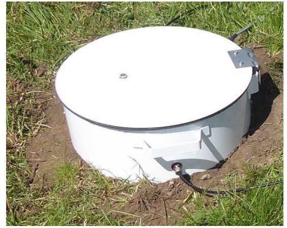
AutoFlux drum during a typical radon flux measurement: accumulation period (1 hour, on the left side) and ventilation period (2 hours, right side).
