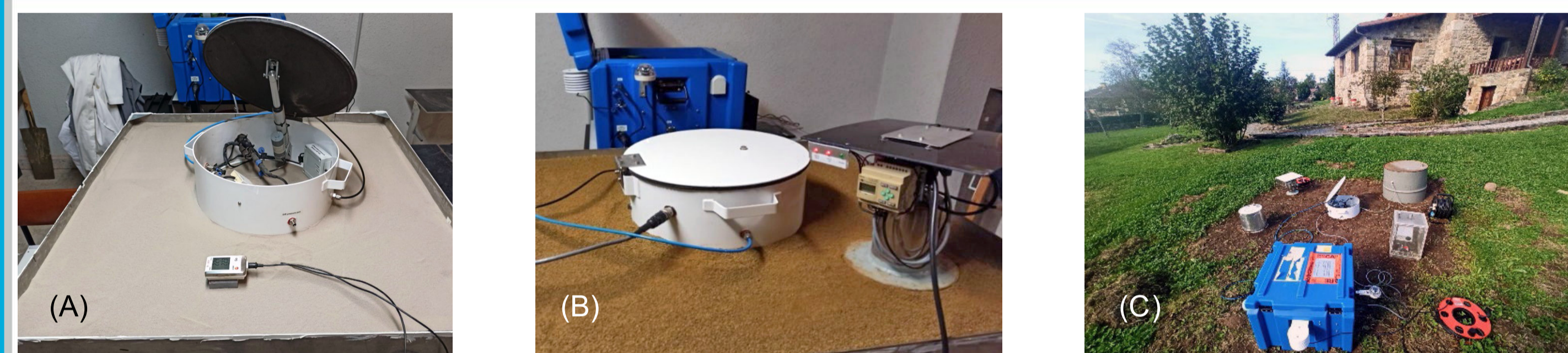
Figure 4: (A) Calibration of flux transfer standard on traceable exhalation bed, (B) intercomparison with transfer standard on exhalation bed, (C) field intercomparison exercise with transfer standard (centre) and different types of flux instruments.
