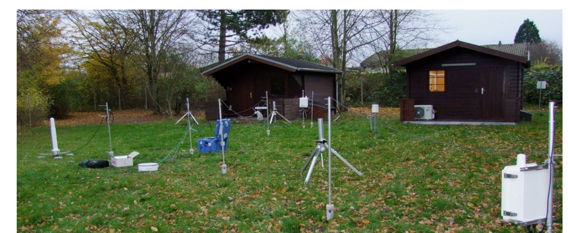
Figure 3. Installation of radon flux systems, dose and spectrometry monitors and soil sensors at the PTB site.
