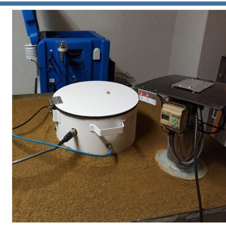
Figure 5. Transfer Standard instrument calibrated and used for radon flux system calibration.
